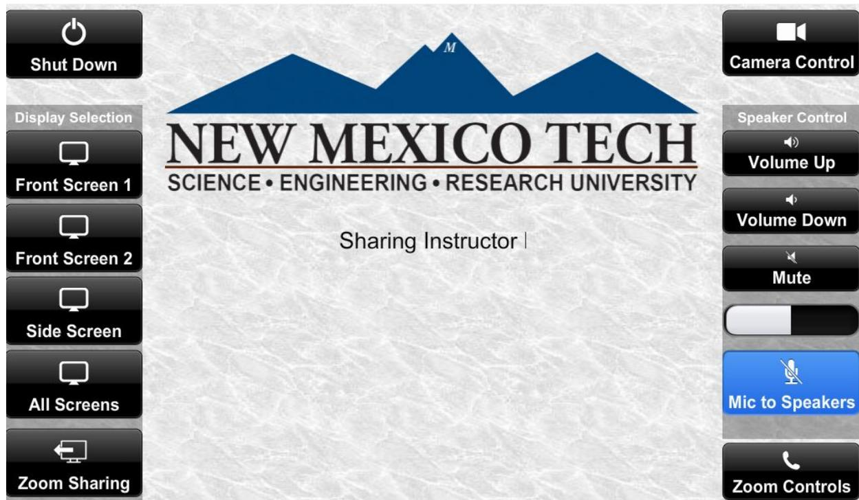
First: Below the volume on the right side of the touch panel is a new button called 'Mic to Speakers'. This button is a way to amplify your voice using the wireless lapel microphone to the room speakers. It is muted by default when the system starts up and will be highlighted in blue as shown. This is to help students hear your lecture even through a mask or face shield.
